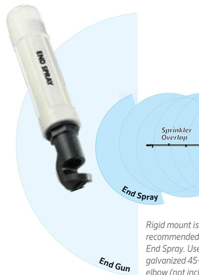
Rigid mount is recommended for the End Spray. Use a 1" NPT galvanized 45-degree elbow (not included). Orient pad of End Spray nozzle to face up.
