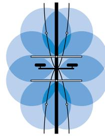
*Booms installed at the towers and on overhangs help reduce wheel tracking regardless of pivot travel direction.*
