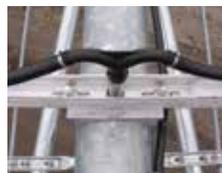
*The Senninger Double Gooseneck attaches to the 3/4" x 4" galvanized nipple through a pre-drilled hole in the aluminum channel and into an existing outlet.*
